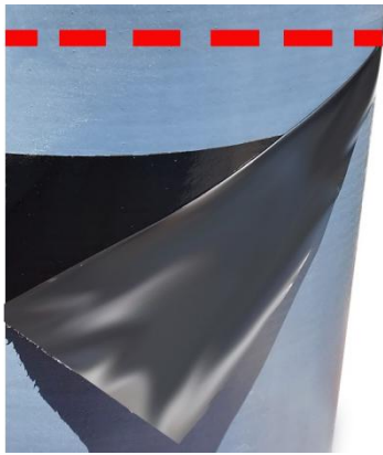
Lower silicon film with overlap flap
